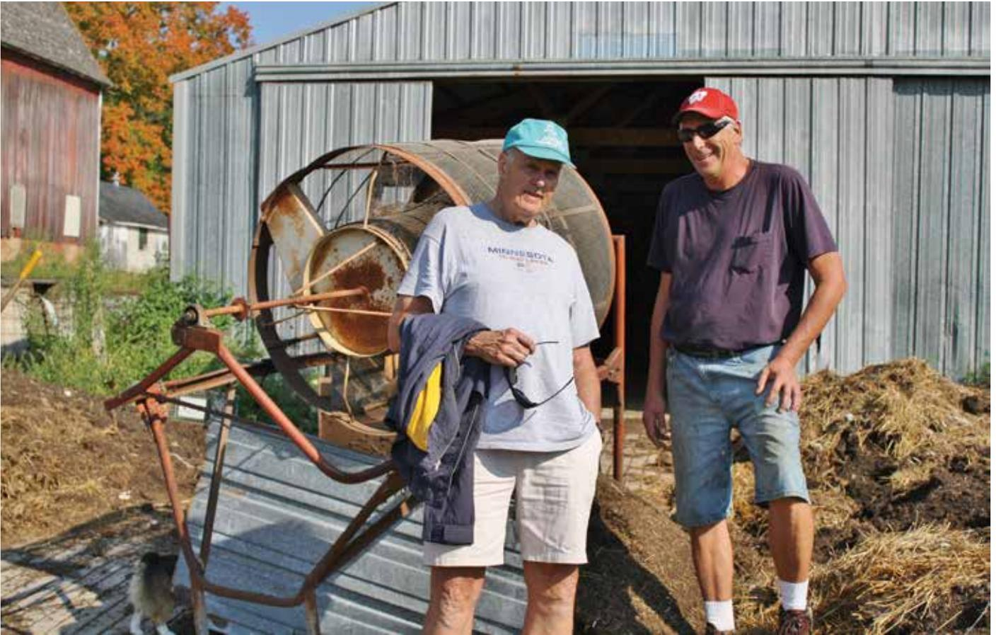
Above: Dan and Ed stand in front of the machine that separates worms from their castings. Right: Here the worms are becoming concentrated after most of the duff has been removed.
